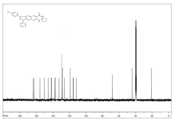
Fig. S17: <sup>13</sup> C NMR Spectrum of 3-(4-chlorophenyl)-7,9-dihydro-8-methyl-6-chloro-1-phenyl-5Hpyrazolo[3,4-d]naphthyrido[2,3-d]pyrimidin-6(5H)-one 10a
