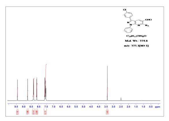
Fig. S5: <sup>1</sup>H NMR Spectrum 6-azido-3-(4-chlorophenyl)-1-phenyl-1H-pyrazolo[3,4-b]pyridine-5carbaldehyde, 5
