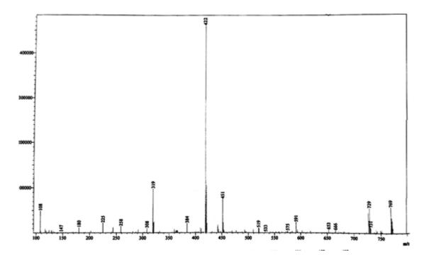
Fig. S2 : Mass Spectrum of N,N-Diphenyl-3-(4-chlorophenyl)-dipyrazolo (3,4-b)pyridine, 3
