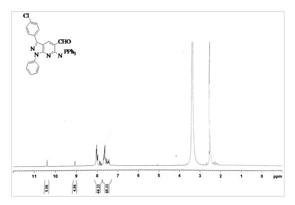
Fig. S4: <sup>1</sup>H NMR Spectrum Triphenylphosphoranylideniamino-pyrazole, 4
