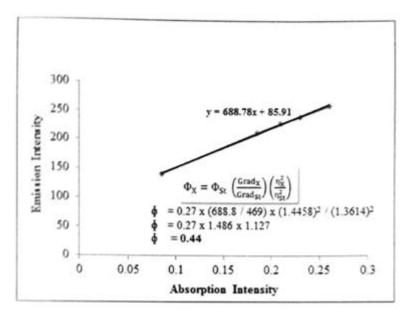
Figure-S23: Graph of emission intensity Vs absorption intensity, calculation of gradient and quantum yield for compound 9h
